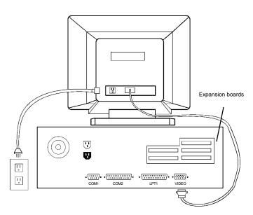
Figure 2-1 Monitor Connections
